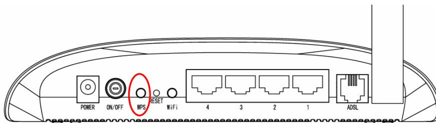
**Step 2:** Press and hold the WPS button of the adapter directly for 2 or 3 seconds.
